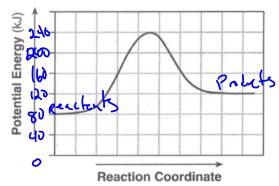
Each interval on the axis labeled "Potential Energy (kJ)" represents 40 kilojoules. What is the heat of reaction?
